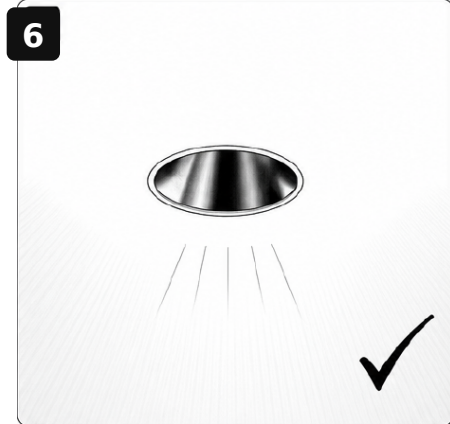
CHECK FLUSH FIT / POWER ON
